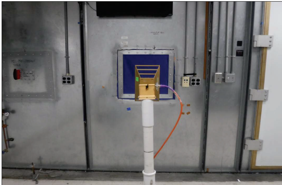
Photograph 8. Shielding Effectiveness, Small Horn EUT Measurement Transmitter, Test Setup
